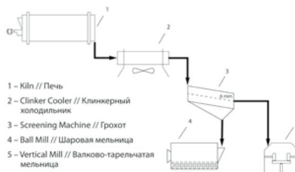
Fig. 8. Diagram in principle of clinker screening with downstream separate grinding
