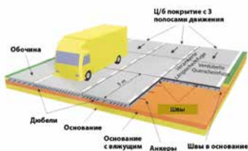
Fig. 3. Schematic view of motorway with cement-concrete pavement
